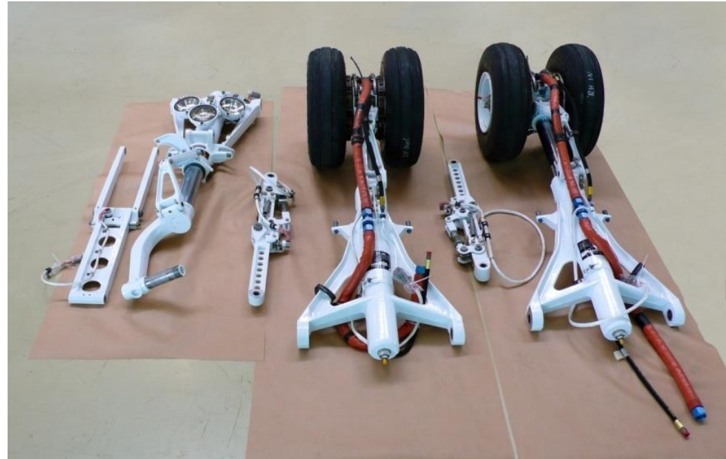
King Air 6-years inspection: Step #9 reassembling of major parts
